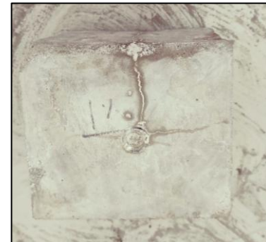
Fig. 7 crack healed after around 28 days
